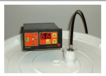
The MC-LEVEL probe is a level meter with microprocessor capable of supplying an analogue signal pro
