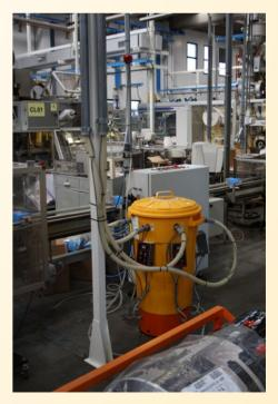
EASY-CHARGE is able to overcome elevation difference. One of the hoses of the 2 channel feeder on the left, has a starting rise of about 4 m (13 ft). Then it runs horizontally for about 12 m (40 ft), and finally it goes down for 3 m (10 ft) to the Hot-Melt system.
