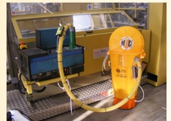
The high consumption of glue of this applicator with a tank of 13kg, required frequent manual filling of glue. Now the automatic feeder EASY-CHARGE maintains the optimal level of adhesive.
